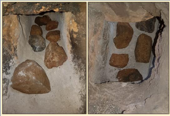
Figure 10: River rock bed installed in the prototypes, 2cm apart (Authors, 2021)
